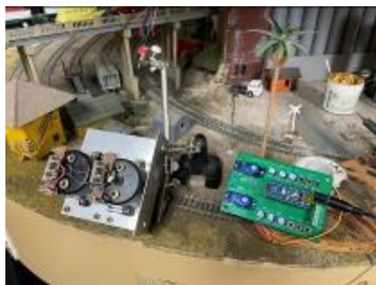
Initial cause or collateral damage? Can't tell for sure. 22-year-old Tomar train order signal control on the left. New MRCS train order signal control on the right, complete with servos managed with an Arduino.
