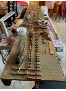
All the ties are in place on this piece. I am building the first switch frog for the Kingfield Switch. This is the switch into Kingfield from the mainline which turned to the left toward Carrabassett and Bigelow.
