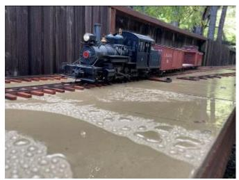
The first train to Kingfield, after a rain shower. No 9 is a stock Bachmann Spectrum Forney, regauged by John Rogers. John Narrowed the wheelset spacing from 45mm to 30mm to properly model 2 foot gauge in 1:20.3 scale.
