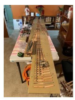
Testing the completed frog on the last switch in this section. The truck I am using to test all the trackwork is scratch-built – and a test in its own right.
