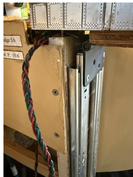
Bridge 5 is now 'up' and trains have the right of way. The bridge was lifted vertically extending the drawer slides, swung out horizontally on the door hinge, and then lowered in place with the door slides collapsing back on themselves.
