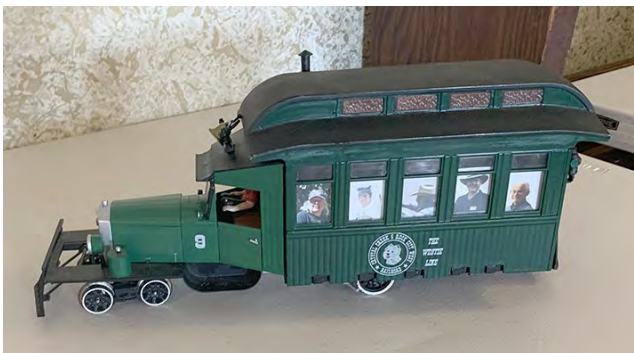
This is a scratch built model rail bus that is battery operated with sound and lights. The pictures in the windows are members of the Redwood Empire Garden Railway Society.
