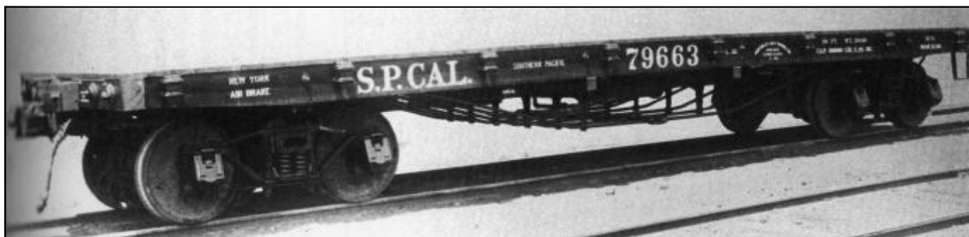
A builder photo of CS-30 car no. 79663. Its completion date was May 28, 1902. The CS-30 cars differed from CS-22 in returning to 36-foot length, but supported 40 tons on six truss rods.
