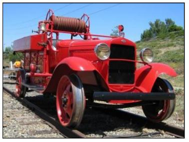
The California State Railroad Museum had this 1931 Ford Model AA Fire Truck on display. This 4 cylinder, 40 hp fire truck was operated by the San Diego & Eastern Railway as MW 1003. It had the ability to refill it's tanks at trackside water tanks and was in service for almost 50 years.
