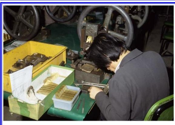
This man is making final preparations to punch holes into the ends of 600 HO scale outside braced open hopper car sides. Each of the steel dies in the yellow tub were created to punch a single hole or series of holes into brass car sides that will be fed one at a time into the rotary punch. You can see a caboose side hanging out of the opening in the punch closest to us. That particular photo etched sheet was fed into the punch, the wheel rotated to actuate the punch, and the window openings
