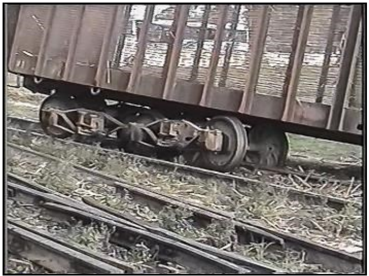
There are no brakes on the sugar cane cars.
