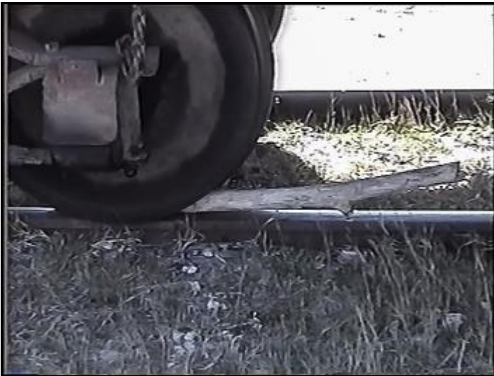
We block or chock cars. This is called "twigging".
