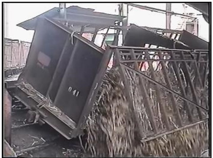
Platform tilts to unload cars.
