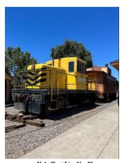
Yolo Short Line No. 50 A GE 50-tonner was Weirton Steel No. 96 and Spreckles Sugar No. 1 (photo: Chip Meriam)
