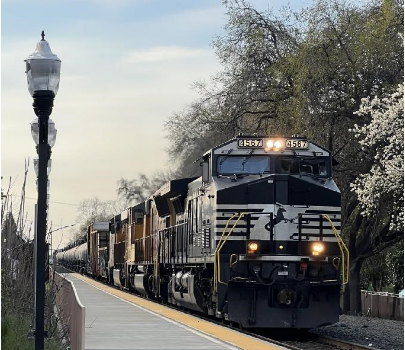
Norfolk Southern #4567, a GE AC44C6M rebuilt May 2022 at Wabtec-Ft. Worth from GE Dash 9-44CW #9371 (original build May 2019). Seen here at 8:03 AM, Saturday, March, 2023, at W. 3rd Steet, running past Chico, CA Amtrak Station.
