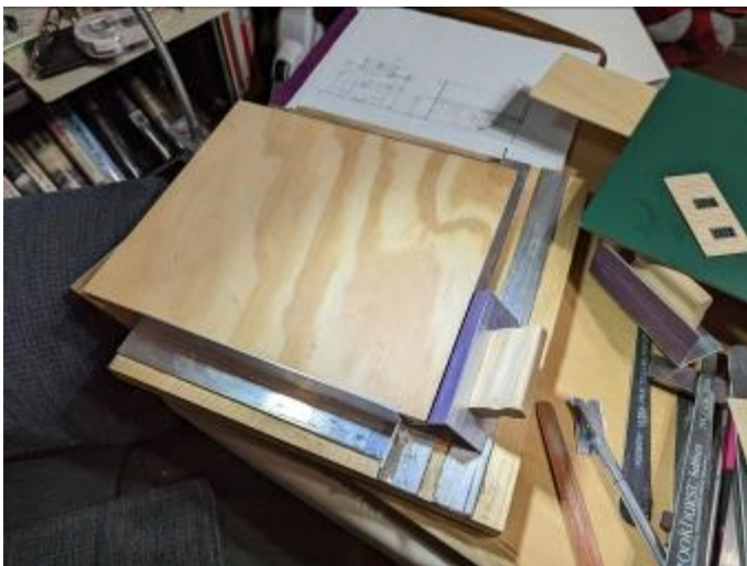
A special jig was constructed to insure that walls met at perfect 45 degree corners. ( MR, August, 2023 )
