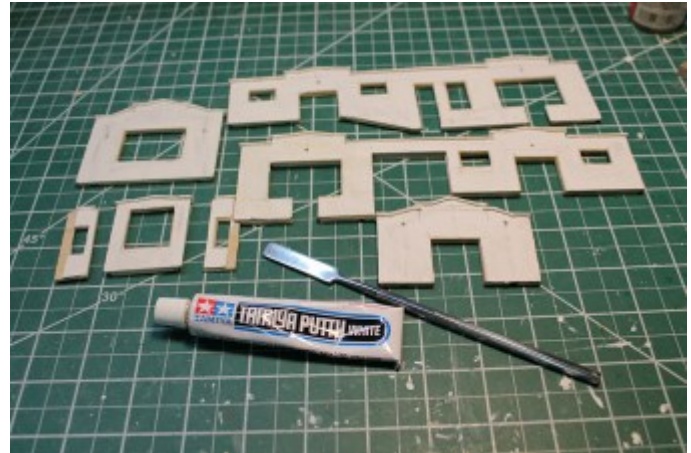
A stucco "brown" coat is simulated with with contour putty.
