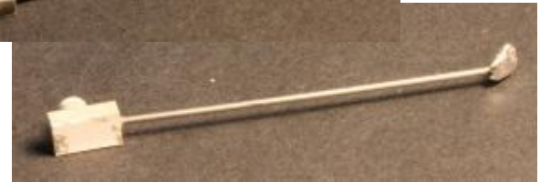
Meter box is assembled from Plastruct styrene rod and styrene rectangular dowel. Conduit is formed from .0374 music wire. Service head is a drop of hot solder applied to the end of the music wire and filed to shape.
