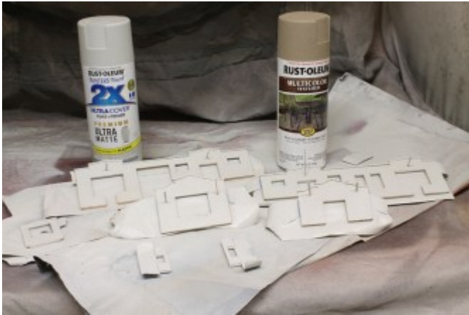
Rustoleum textured spray paint is applied to create the stucco texture coat. The final (color) coat is a light, flat gray primer.
