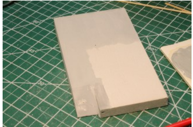
Finished slab foundation cast in Plaster of Paris. Ramp is formed by filing with a large mill bastard file and finished with emery boards.
